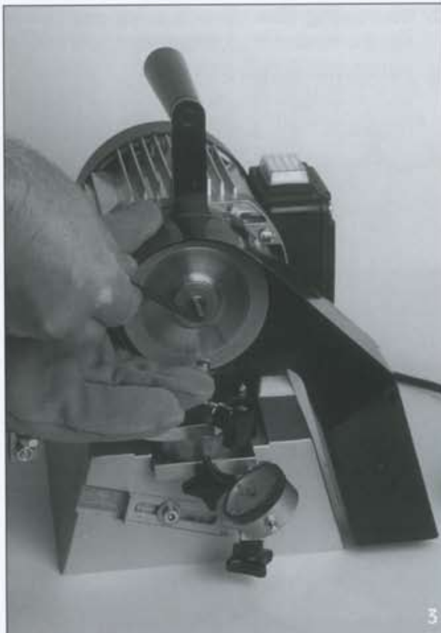
Change of the diamond disk: Main switch is "0" = "off". Pull plug!
