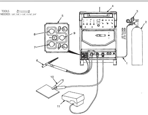
**1** Gas Hose With 5/8"-18 Right-Hand Male Thread Fittings at both ends
