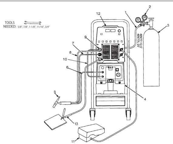
**1** Gas Hose With 5/8"-18 Right-Hand Male Thread Fittings at both ends
