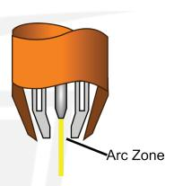
The welding arc transfer is gentle, consistent and accurate, allowing for welding of thin sheets, fine wire and miniature components.
